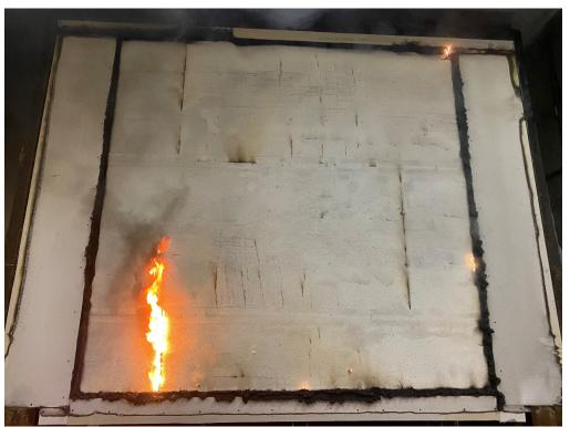
Figure 6: The exposed face after the fire test.
