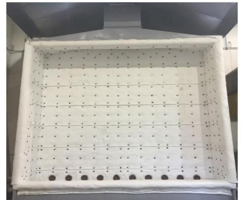
Figure 1: Full Scale Furnace
