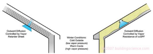
In colder temperatures, when spray foam has been installed at a sufficient thickness, the foam provides the first condensing plane.
