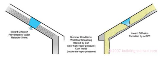
In warmer temperatures, spray foam allows the assembly can still dry to the inside because the spray foam is a vapour retarder rather than a pure vapour barrier.
